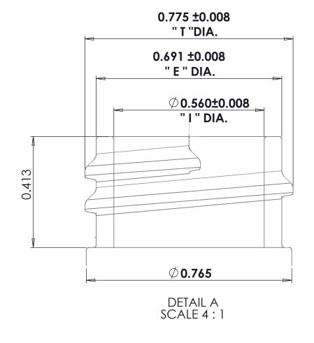
Rev. B tolerance changed from 0.028 to 0.039 on overall height , added tolerance on I dimension. 01/04/2018
